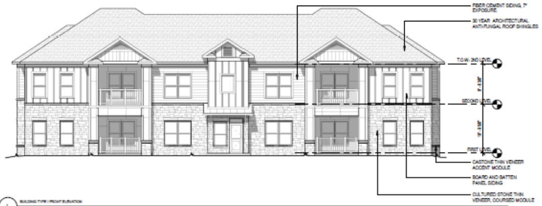
3 BUILDING TYPE / FRONT ELEVATION 1/8" = 1'-0"
