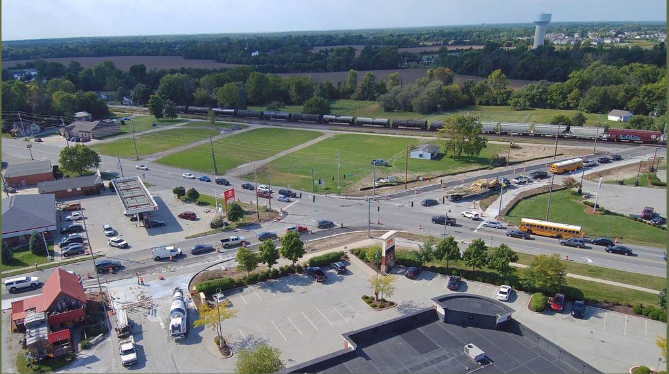
Right turn lanes made at the intersection of CR 600 West and Broadway have helped provide a smoother flow of traffic.
