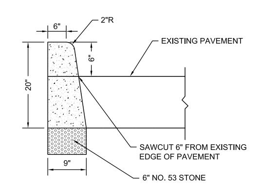
**CONCRETE CURB (BARRIER)** SCALE: NONE
