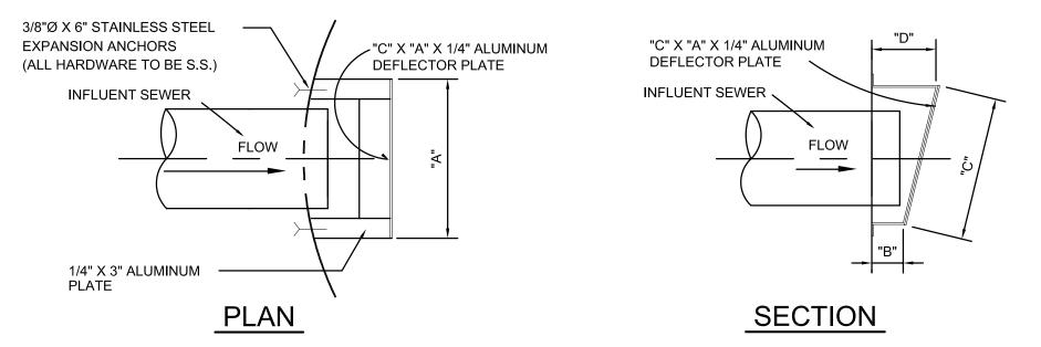
ALL SURFACES CONTACTING CONCRETE SHALL HAVE A BITUMINOUS COATING
