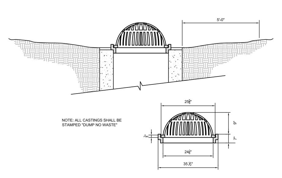
BEEHIVE GRATE CASTING WITH FRAME - NEENAH R-2560-E2
