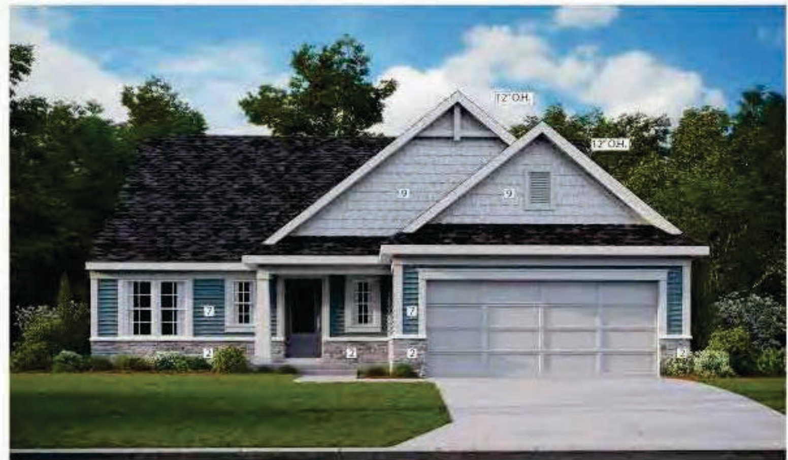
KEATON - WESTERN CRAFTSMAN W/ STONE STONE (2) = 27% VINYL HORIZONTAL SIDING (7) = 37% HARDI-PANEL SHAKE SIDING (9) = 27% TOTAL MASONRY = 63%
