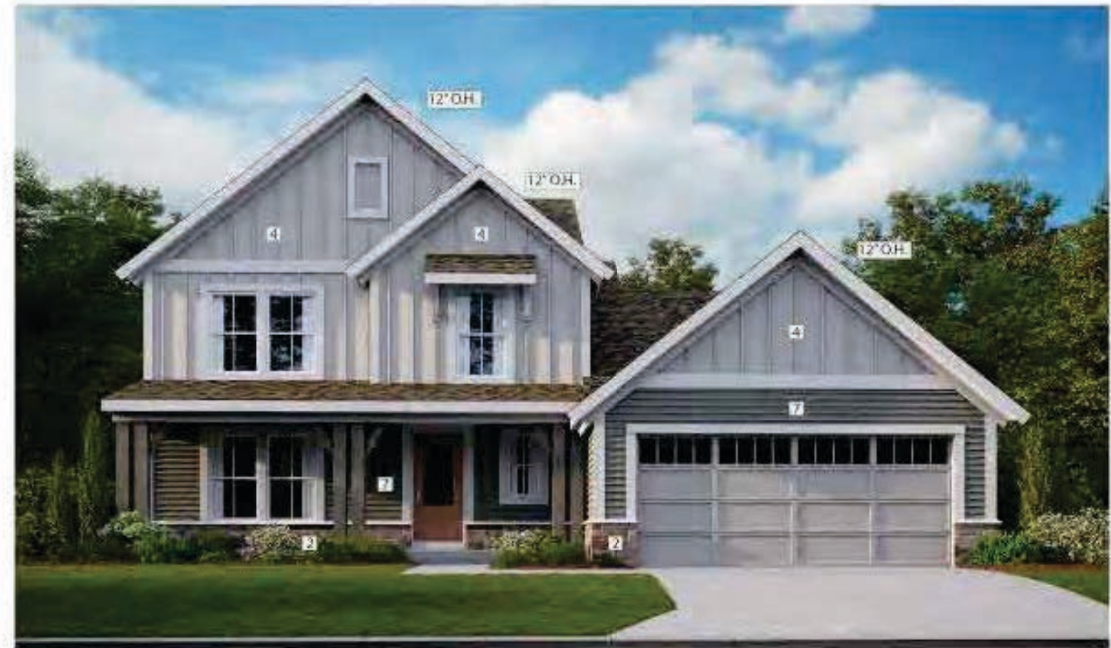
CHARLES - MODERN FARMHOUSE W/ STONE STONE (2) = 14% HARDI-PANEL (4) = 57% VINYL HORIZONTAL SIDING (7) = 35% TOTAL MASONRY = 65%
