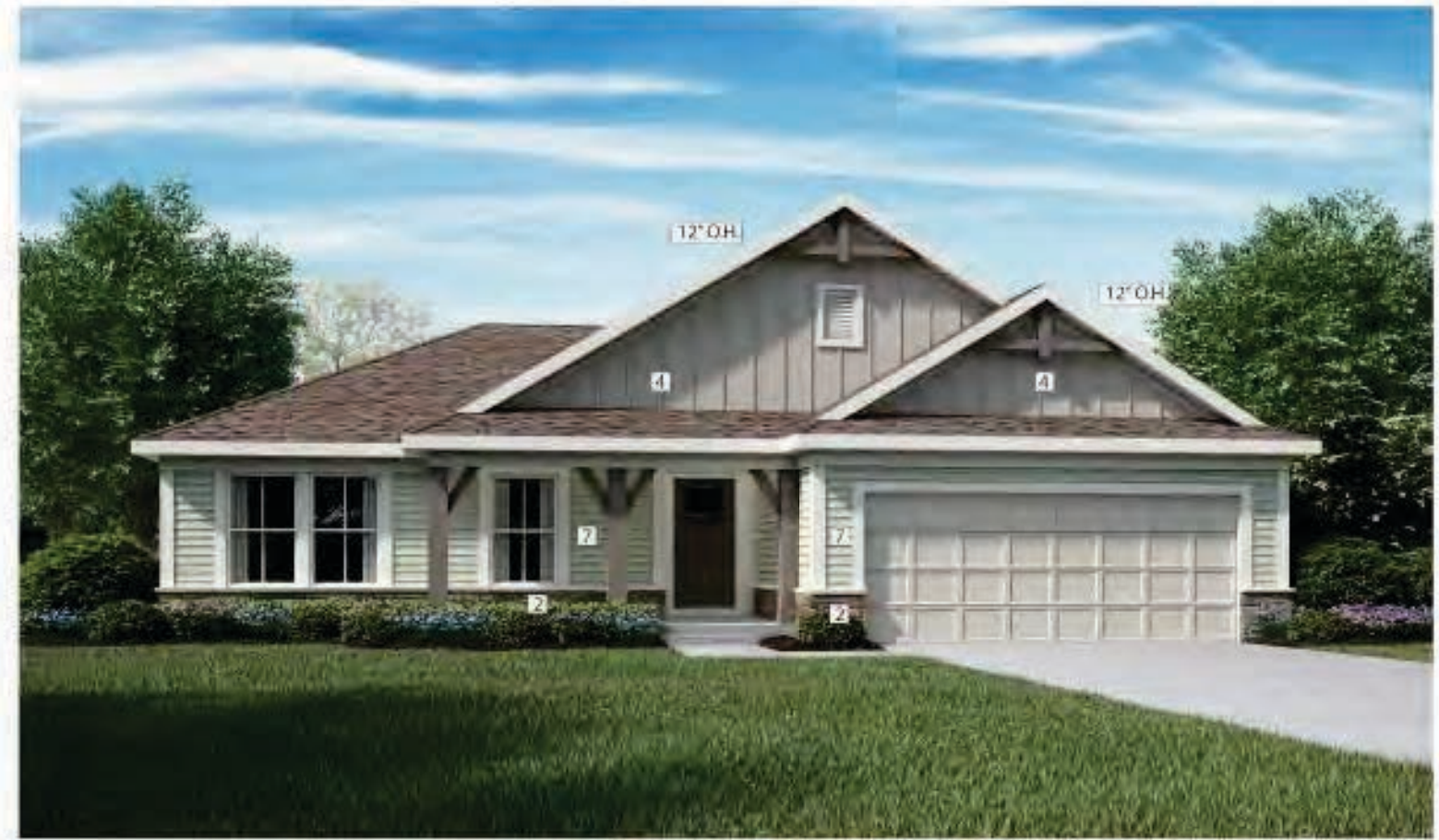
SPRINGFIELD - MODERN FARMHOUSE W/ STONE STONE (2) = 22% HARDI PANEL (4) = 41% VINYL HORIZONTAL SIDING (7) = 37% TOTAL MASONRY = 63%
