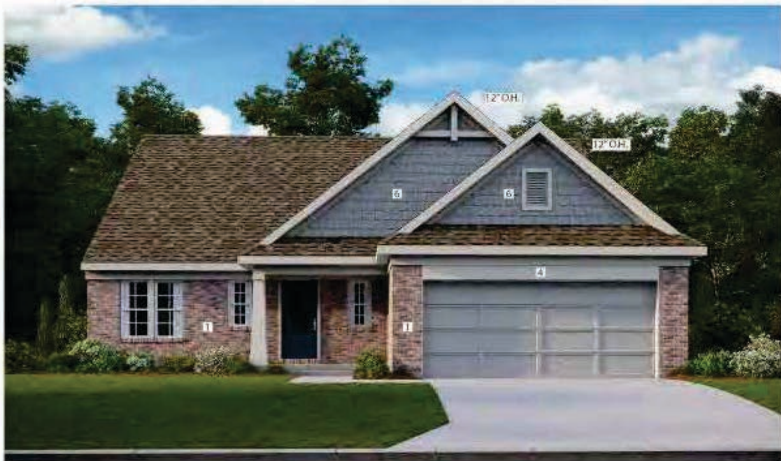
KEATON - WESTERN CRAFTSMAN W/ BRICK BRICK (1) = 63% HARDI-PANEL (4) = 5% VINYL SHAKE SIDING (6) = 32% TOTAL MASONRY = 68%
