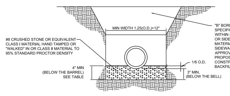
"B" BORROW AS DEFINED BY CURRENT INDOT SPECIFICATIONS WHEN TRENCH OPENING ENCROACHES WITHIN 5' OF AN EXISTING OR PROPOSED PAVED AREA OR SIDEWALK. NATIVE BACKFILL OR OTHER APPROVED MATERIAL SHALL BE USED OUTSIDE OF PAVED AREA OR SIDEWALK BACKFILL LIMITS. NATIVE BACKFILL OR OTHER APPROVED BACKFILL MATERIAL MAY BE USED UNDER PROPOSED SIDEWALKS PROVIDED SIDEWALKS ARE CONSTRUCTED 6 MONTHS (MINIMUM) AFTER BACKFILLING OF TRENCH.
