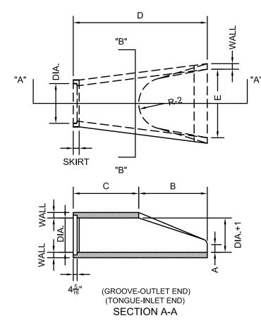
PRECAST CONCRETE END SECTION DETAIL NOT TO SCALE
