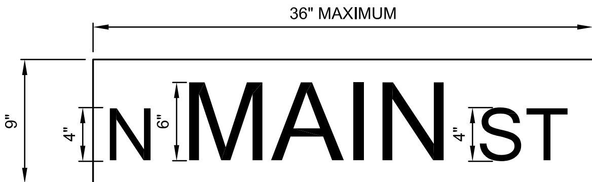
ROAD NAME SIGN DETAIL SCALE: NONE
