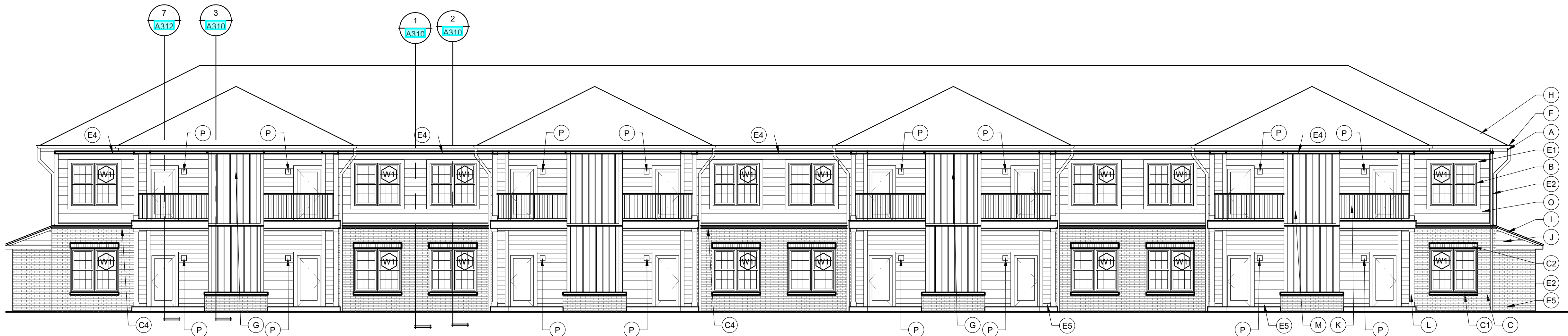
2 ELEVATION - TYPE A - REAR OVERALL Scale: 1/8" = 1' - 0"
