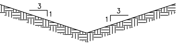
TYPICAL SWALE SECTION (MAX. SIDE SLOPE - 2:1)
