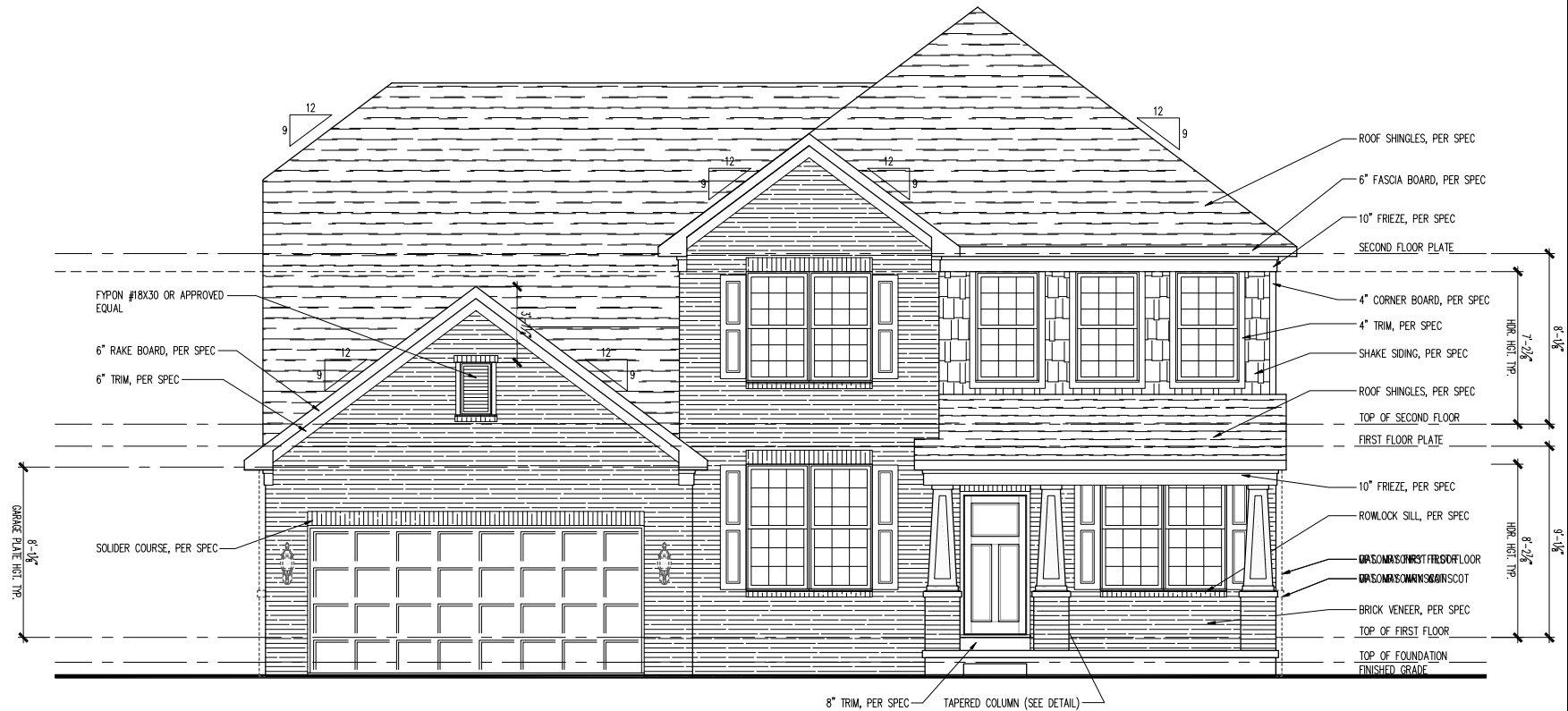
FRONT ELEVATION SCALE: 1/4" = 1'-0"
