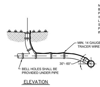
NOTE: A MINIMUM 6" DIA PIPE TYPE I CLEAN OUT SHALL BE INSTALLED 3' AWAY FROM BUILDING. A THREADED PLUG SHALL BE USED TO ENSURE 100% WATERTIGHTNESS. FOR LATERALS GREATER THAN 100 LF AS MEASURED ALONG THE PIPE, TYPE II CLEAN OUTS SHALL BE INSTALLED AT THE STREET RIGHT-OF-WAY OR PROPERTY LINE AS APPLICABLE AND AT 100 FOOT INCREMENTS AS APPROPRIATE.
