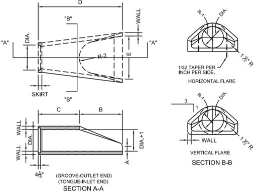
**PRECAST CONCRETE END SECTION DETAIL**
