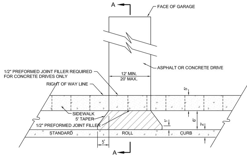
1. CROSS HATCHED AREAS SHALL BE EITHER 6" PLAIN CONCRETE OR 1" SURFACE ON 2" BITUMINOUS BASE ON 4" #53 COMPACTED AGGREGATE BASE, EXTENDING TO THE SIDEWALK OR R/W LINE WHICHEVER IS NEAREST TO THE ROADWAY.
