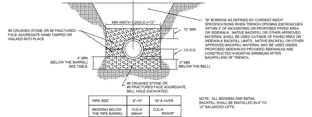
**FLEXIBLE PIPE (HDPE & PVC) TRENCH DETAIL**
