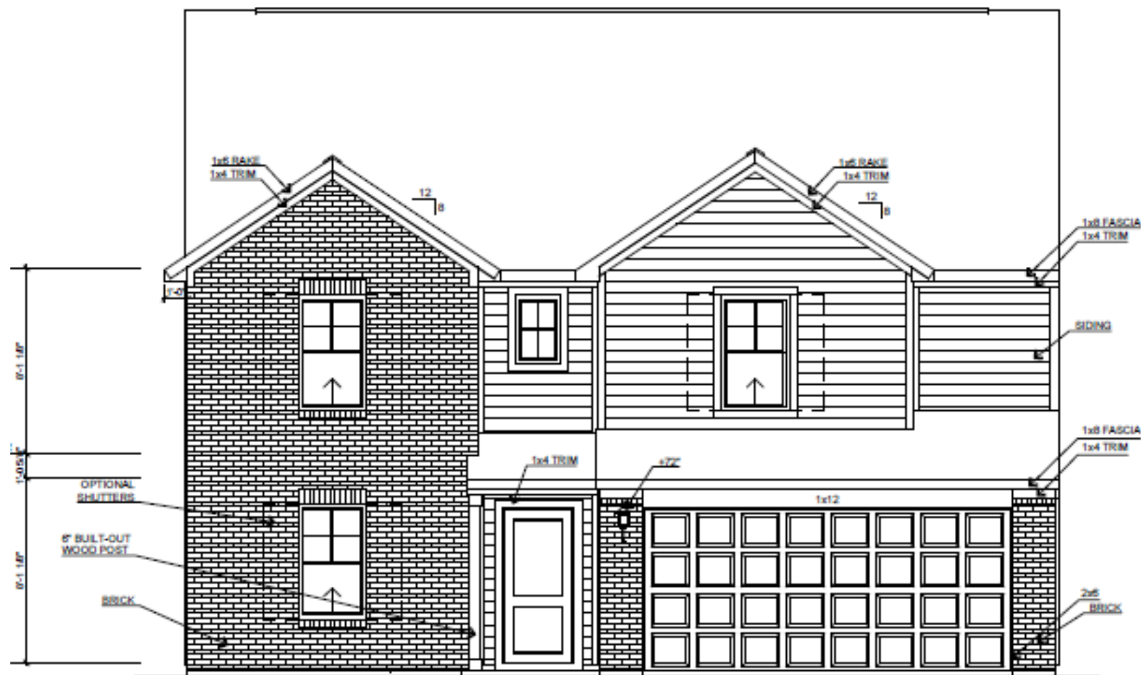
FRONT ELEVATION A - BRICK FRONT - C
