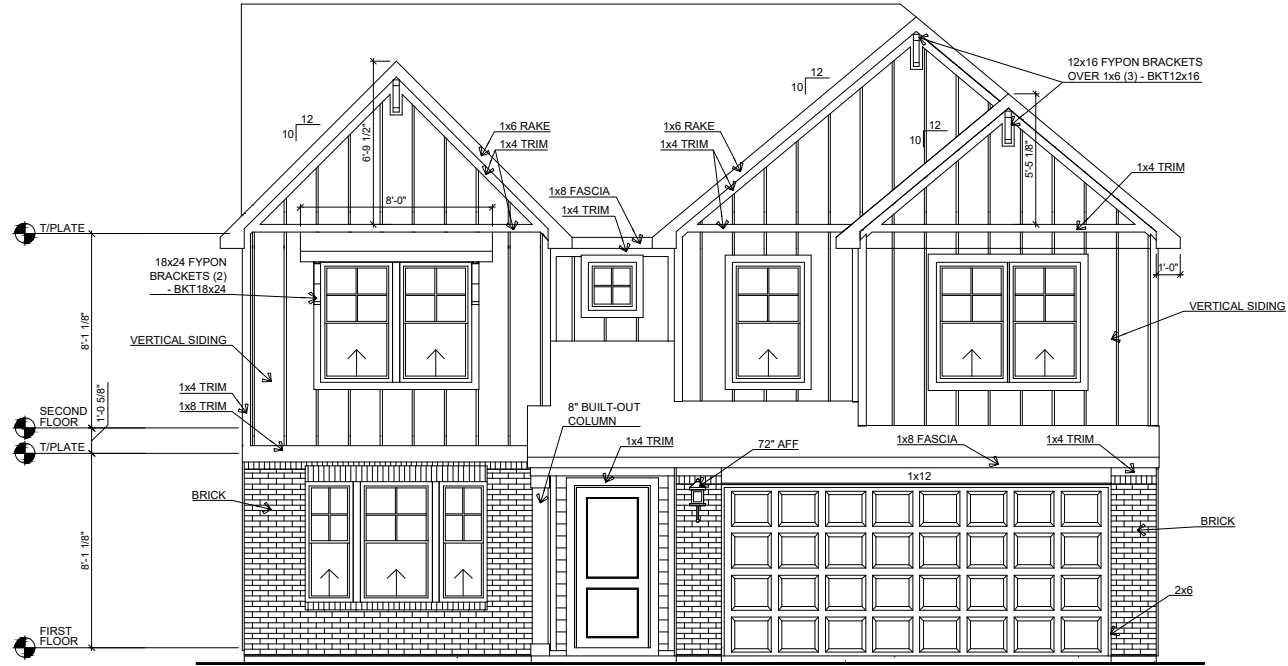
✓ FRONT ELEVATION E - SLAB - BRICKFRONT C SCALE: 1/8"=1'-0"
