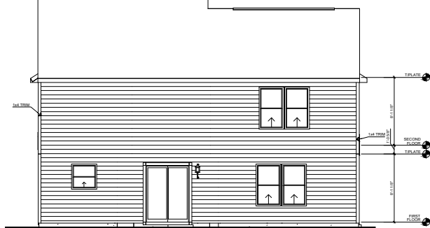
REAR ELEVATION - SLAB
