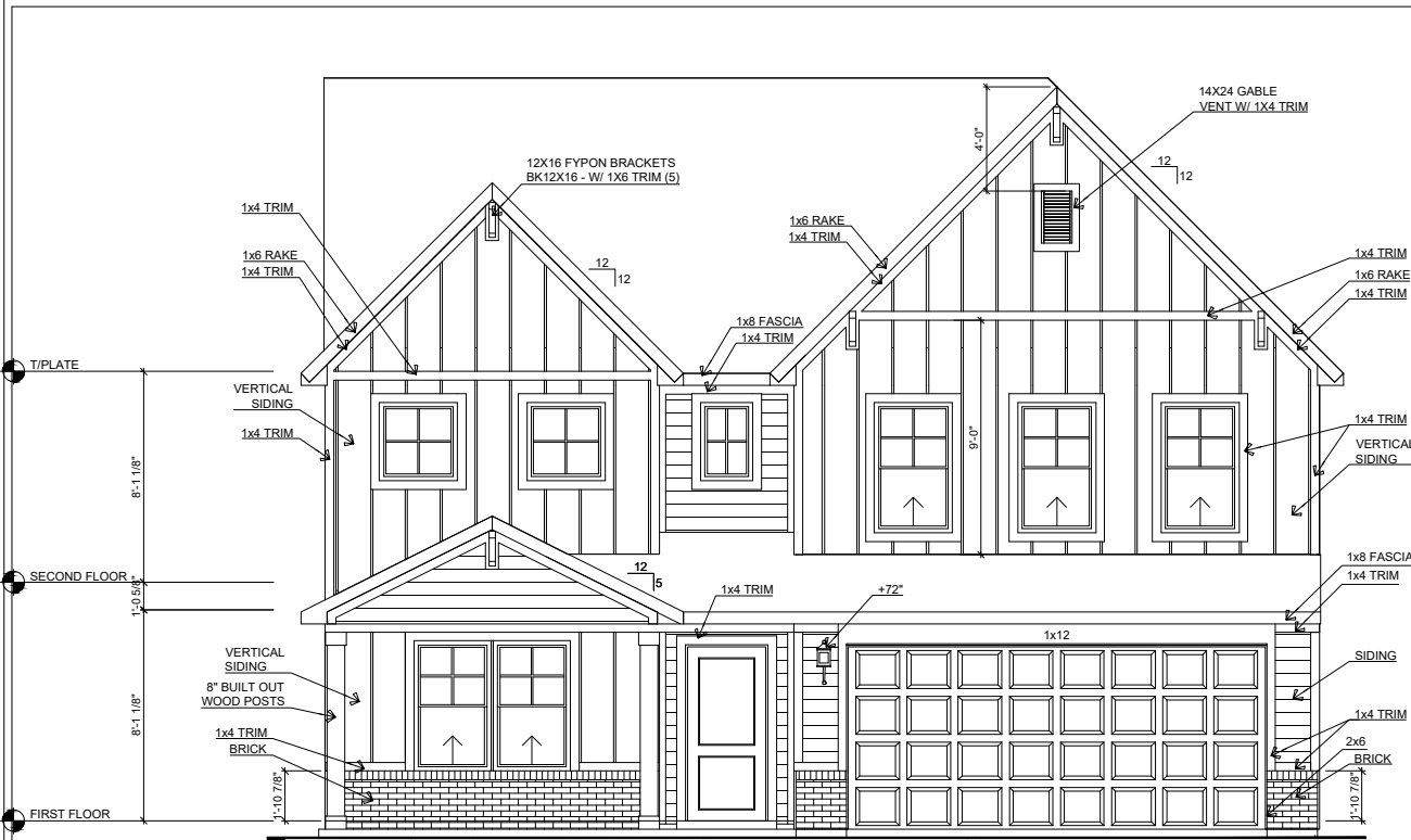
FRONT ELEVATION E - BRICKFRONT A
