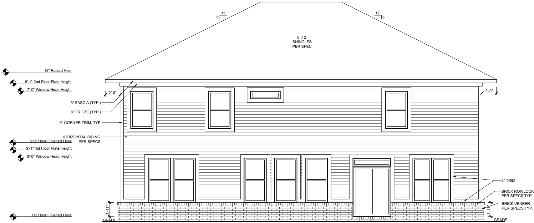
REAR ELEVATION-PRL SCALE: 1/8"=1'-0" (11"x17" SHEET SIZE) SCALE: 1/4"=1'-0" (24"x36" SHEET SIZE)
