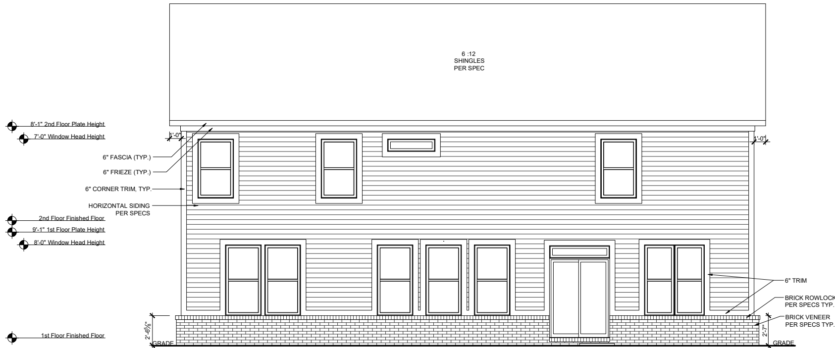
REAR ELEVATION-FHL SCALE: 1/8"=1'-0" (11"x17" SHEET SIZE) SCALE: 1/4"=1'-0" (24"x36" SHEET SIZE)
