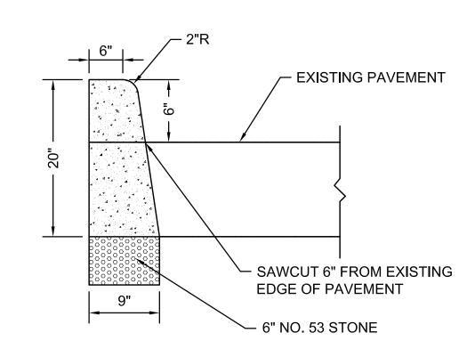
CONCRETE CURB (BARRIER) SCALE: NONE
